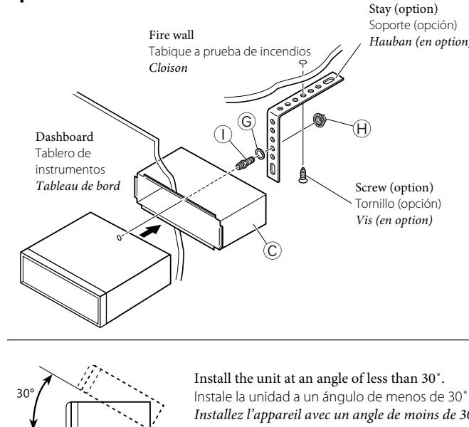
Install the unit at an angle of less than 30°.
